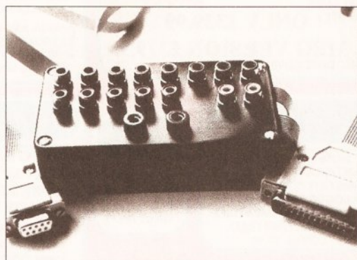
Switchsoft's I/O Port showing the two 'D' connectors going to the parallel port and joystick ports. The phono connectors provide facilities for an assortment of applications
